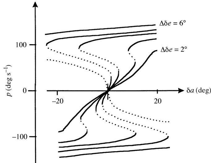
Figure 3. Inertia coupling: steady roll rate versus aileron deflections: —, stable; ---, unstable divergent.
