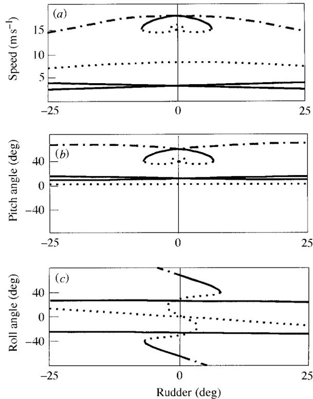
Figure 5. Equilibria of a submarine model. —, Stable; ---, unstable divergent; - · - ·, oscillatory unstable.
