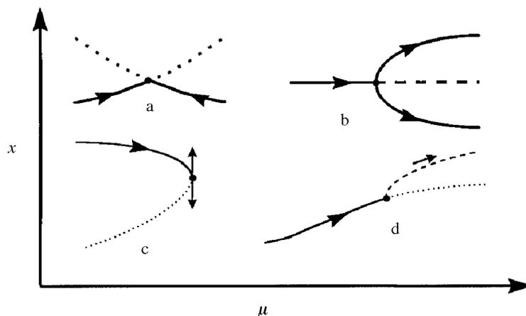
Figure 17. Examples of possible crossing bifurcation and limit points during quasi-stationary behaviour.
