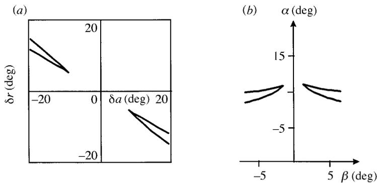
Figure 2. Spiral bifurcation in aileron-rudder plane.
