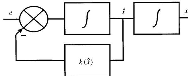
Figure 12. Controlled unstable second-order dynamic system.
