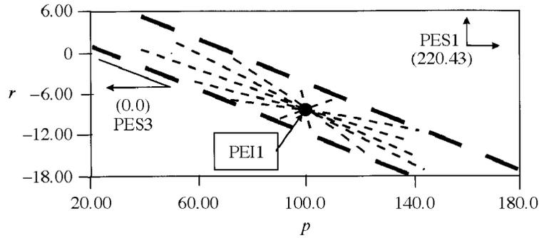
Figure 16. Projection in the (roll rate, yaw rate) plane of the boundary of the domain of stability. PES1 and PES2 are stable equilibrium points while PEI1 is an unstable one.
