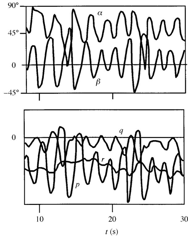
Figure 11. Motion on a toroidal surface for  $\delta_a = -10^\circ$ .
