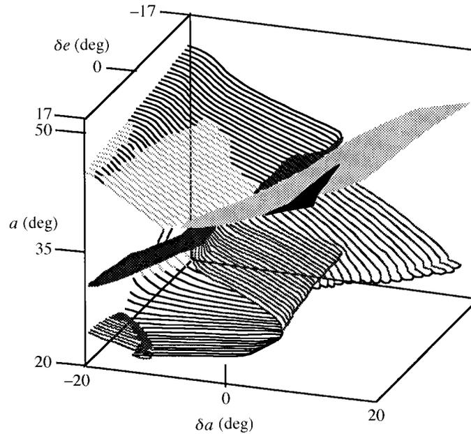
Figure 6. Equilibrium surface projection in a characteristic subspace (aileron, rudder, incidence).
