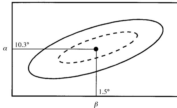
Figure 14. Fixed point and periodic orbits for a typical stabilized combat aircraft. —, stable orbit; ---, unstable orbit.
