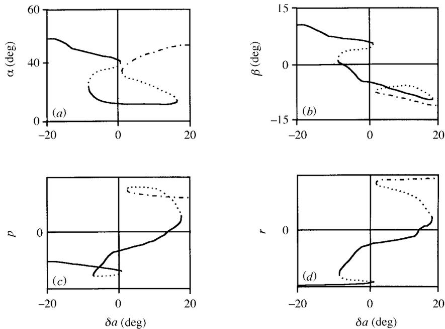
Figure 7. Equilibrium curve for  $\delta_r = 17^\circ$ : —, stable;  $\cdots$ , unstable divergent;  $---$ , oscillatory unstable.
