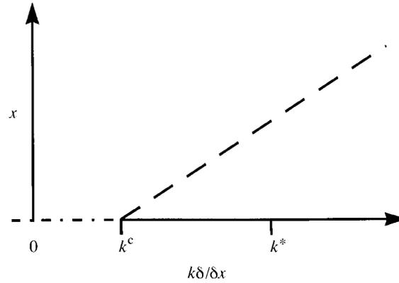
Figure 13. Amplitude of the steady solutions as a function of the nonlinear control gain: —, stable; ---, unstable; - · - ·, oscillatory unstable.
