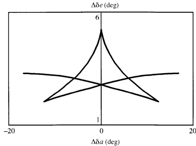
Figure 4. Inertia coupling: bifurcation surface in aileron-elevator plane.
