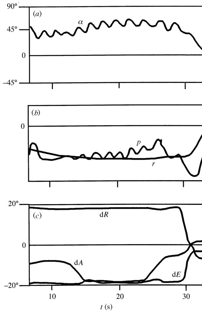
Figure 9. Quiet left spin for  $\delta_a = -4^\circ$ .
