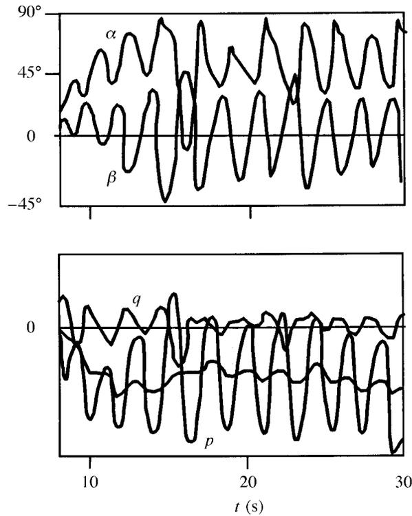
Figure 10. Regular agitated spin for  $\delta_a = -10^\circ$ .
